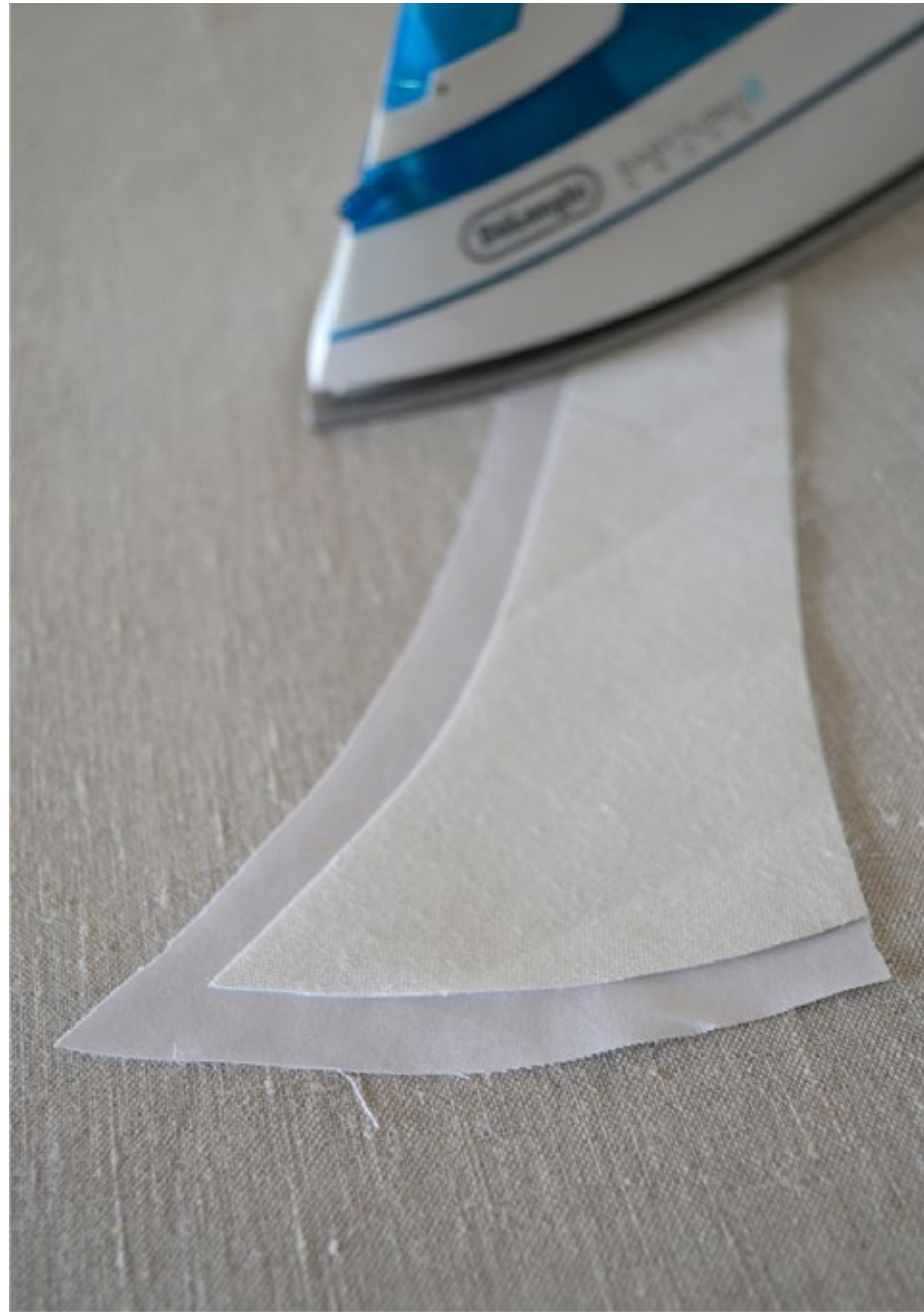
6) Use the iron to fuse the interfacing to the collar. (It takes about 12 seconds).
